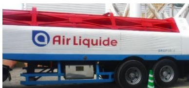
Storage tank for hydrogen fuel
