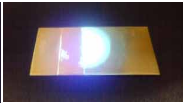
Photo of the illuminated specimen (under a fluorescent lamp in the room) UV LED (365 nm) 30 mW/cm 2
