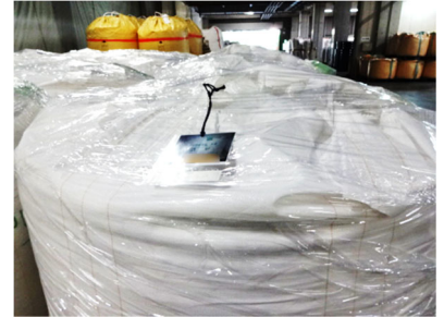
Raw material attached with an RFID tag
