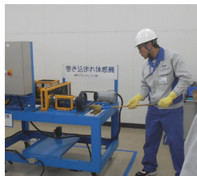
Experiencing getting caught in a revolving belt and roller at the Yokohama Technical Center
