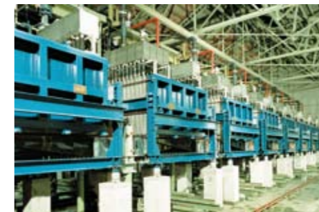
Ion-exchange electrolysis equipment for manufacturing caustic soda and chlorine.
