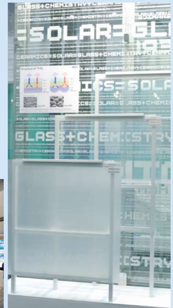
TCO glass Substrate – A high-quality coating used to boost the performance of solar cells.
