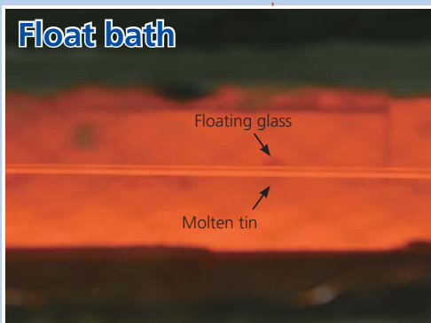
Glass and molten tin in a float bath
