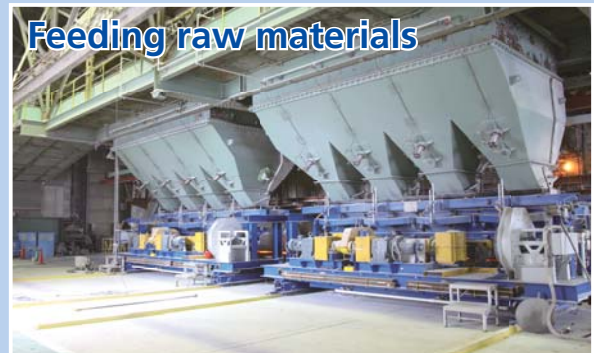
Raw materials are put into a huge melting furnace and are heated by a powerful burner
