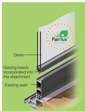
"PairPlus™" is glass that incorporates an attachment frame into double glazing so that the unit can be installed in a single glazing sash used in an existing house.
