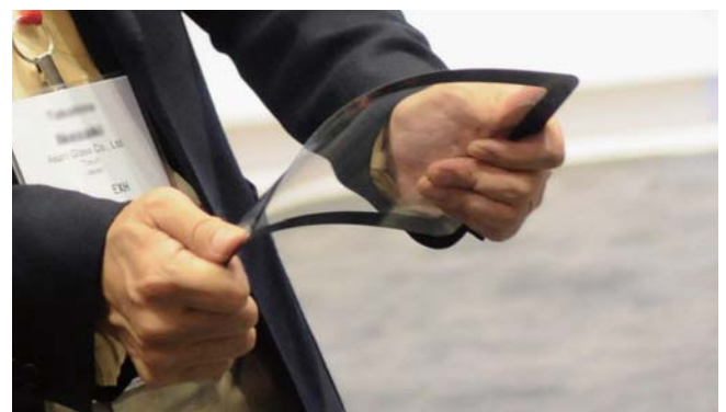
Shock and scratch resistant "Dragontrail™," a specialty glass designed for chemical strengthening
