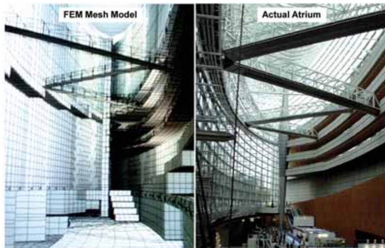
Fig. 8 Indoor view of the actual atrium and the FEM mesh model.
