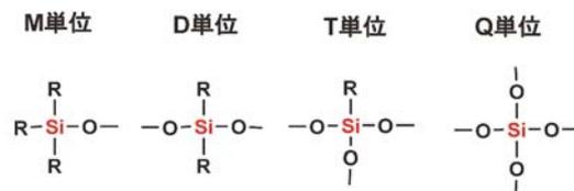
Fig. 1 Unit structures of silicone
