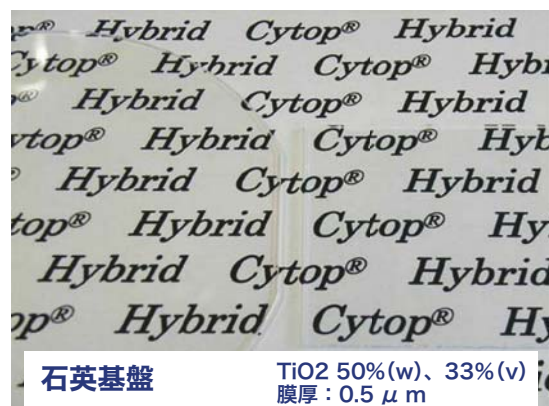
Fig.4 Transparent membrane of the CYTOP® A-type composite including the content of 50 wt. % (33vol.%) of titania.
