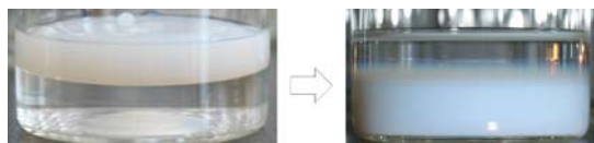
Fig.3 Before (left) and after (right) separating titania nano particles from the acidic sol in CYTOP® A-type solution.
