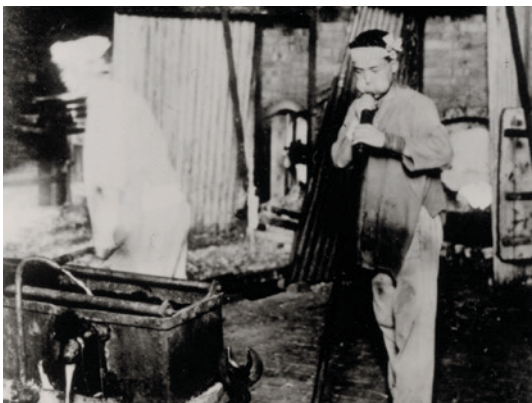
Mass production of flat glass using a Belgian method of producing glass with hand-blown cylinders begins for the first time in Japan (1909)
