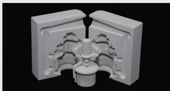
Brightorb™ modeled with a 3D printer
