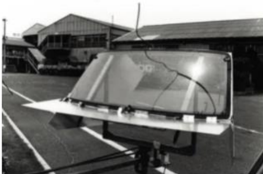
A scene from a glass antenna performance test by AGC (1980s)
