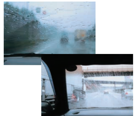
Windshields without water-repellent finishing (top) and with water-repellent finishing (bottom), showing water drops being repelled naturally to ensure a clear view.
