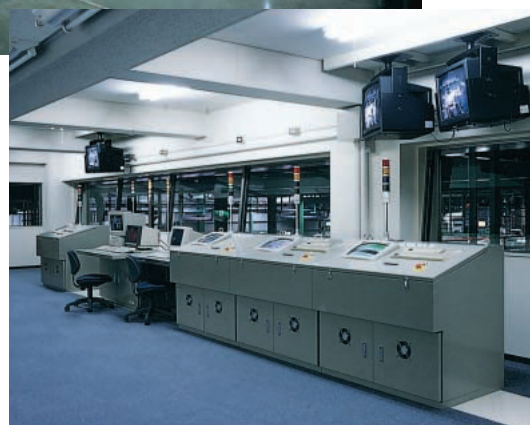
The automated fabrication line equipment for automotive glass, with the operation being monitored collectively in a separate fabrication line monitoring room.
