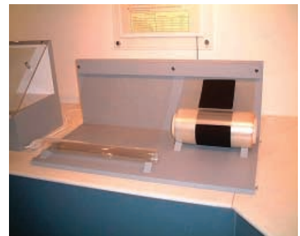
The "membrane-electrode assembly" is produced by integrating membrane and electrocatalysts. This part is sandwiched by separators and then piled repeatedly in multilayers makes an assembly called a stack. This stack, when combined with peripherals, makes a fuel cell system.
