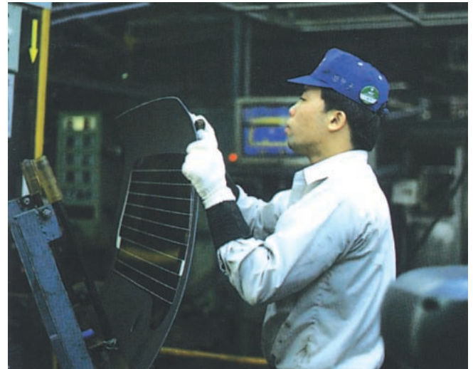
The manufacture of automotive glass is almost completely automated. However, human eyes are still more reliable in inspecting for defects such as scratches.
