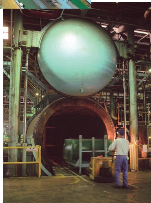
Autoclave (pressure device), a cylinder facility with a large hemispheric door. Two sheets of fabricated glass with film laminated are put inside the autoclave for bonding under high pressure. The autoclave is 4 m in diameter.
