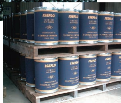
Example of 50 kg fiber drum of "ISEFLO": About 70% of iodine products are exported in this container to different countries.
