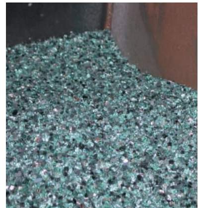
When recycling tempered glass, it is necessary to separate cullet into black cullet and transparent cullet using separation equipment.
