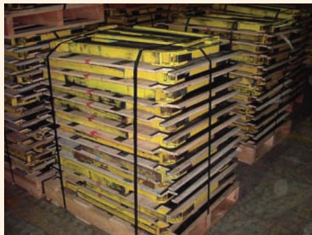
Steel container easy to fold. The steel material can be repeatedly used and can be folded on return, contributing to energy saving and conservation of resources.
