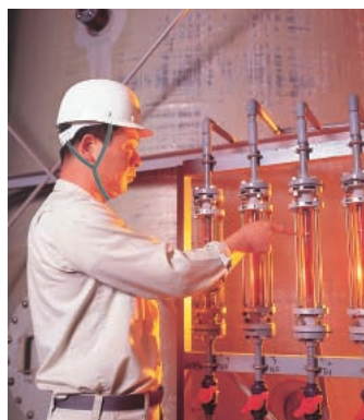
Left: Manufacturing line for cobalt compounds used for batteries of personal computers and cell phones Top: CoO (Cobalt monoxide) Bottom: Co(OH) 2 (Cobalt hydroxide)
