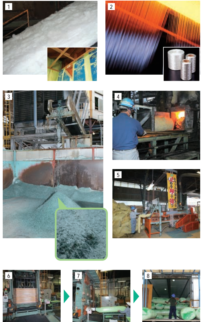
1. Manufacture of glass wool and installation of heat insulation material 2. Manufacture of long glass fiber and product roving 3. Cullet from the manufacturing process is automatically discharged outside to be recycled into raw material 4-5. Defective glass wool is made into cullet, with fragments cut and made into other products to minimize production loss. 6-8. Finished insulator is compressed before packaging, contributing to improving distribution efficiency and reducing energy consumption.
