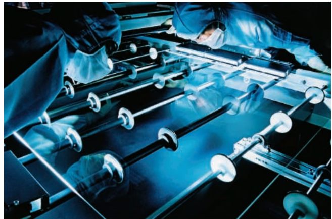
View of final inspection of glass substrate for plasma display panels. Bubbles with diameters as small as 0.1 mm and minute scars are carefully screened out.
