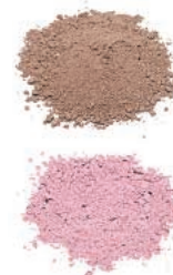
Left: Manufacturing line for cobalt compounds used for batteries of personal computers and cell phones Top: CoO (Cobalt monoxide) Bottom: Co(OH) 2 (Cobalt hydroxide)
