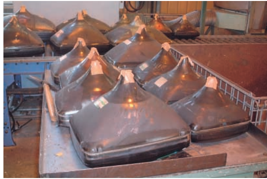
Disposed-of CRT glass collected for recycling will be crushed at the intermediate treatment enterprise into cullet form.
