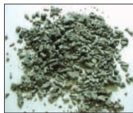
Slag after drying, turned into raw material for glass
