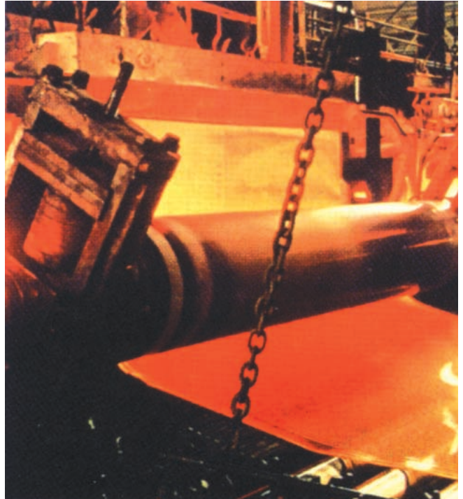
A net is clipped between two heated sheets of flat glass to produce the wire glass for construction. The melting temperature reaches 1500°C or over, but glass here is kept under 900°C.
