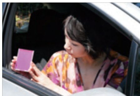
A test with a UV checker, which reacts when exposed to ultraviolet rays.
