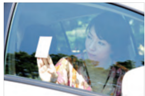
The UV checker turned purple when the window was opened; when shielded by UV Verre Premium™, the color fades away.
