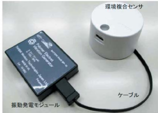
Fig.12 Picture of surrounding environment information sensor powered with vibration electret generator module.
