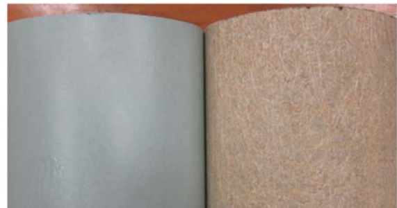
Fig.1 The specimen of outdoor weathering test. (left : before, right : after) ※Place : Saitama pref., Elapsed time : 33years
