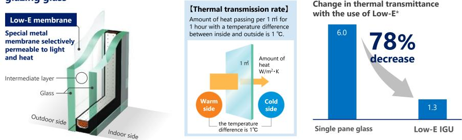
\* Comparison of thermal transmittance between 3 mm float glass and gas-filled Low-E IGU
