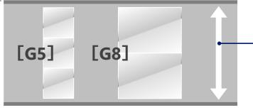
The float process has greater effective width, which allows the production of a multiple number of large-sized glass substrates at a time.
