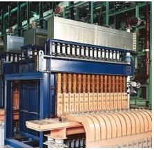
Electrolysis system, using AGC's ionexchange membrane (Flemion™)
