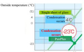
Assuming the room temperature is 20°C and the interior humidity is 50%, condensation starts to occur with a single sheet of glass when the outside temperature is 4°C. On the other hand, Pairplus<sub>TM</sub> ecoglass prevents the glass surface from causing condensation until the outside temperature decreases to -23°C.
