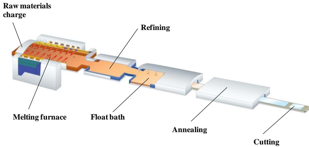
The float process enables efficient manufacturing of large, flat sheets of glass by floating liquid glass on molten tin.
