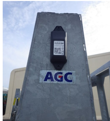
Logistics tracker mounted on the pallet
