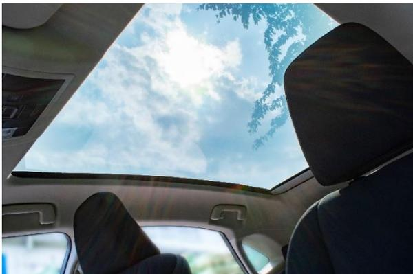
When a voltage is applied to the film, the special material aligns in the same direction, becoming transparent as light is able to pass through. This provides a wide sense of openness.
