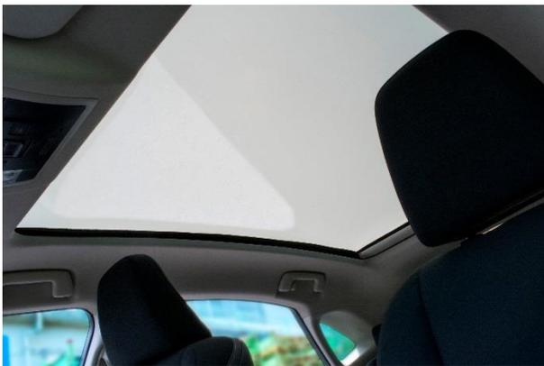
Once arranged into a random pattern, the special material diffuses light from the outside to turn opaque and reduce glare.
