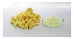
Argyrodite Sulfide-based solid-state electrolyte by AGC's proprietary method
