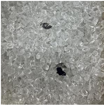
Cover glass from a solar panel that was collected in a crushed condition, which requires removal of foreign objects prior to recycling.
