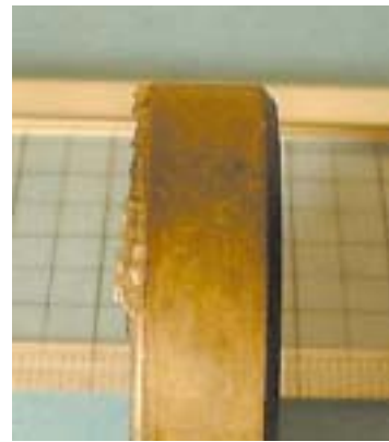
Fig. 2 An example of glass stuck on plunger mold.
