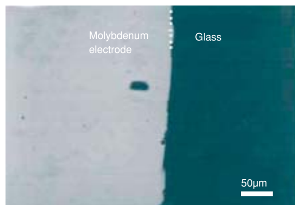
Fig. 4 BEM image of molybdenum/glass interface after dipping in the glass melt without \text{Sb}_2\text{O}_3 at 1450°C for 24h with rotation of the crucible.
