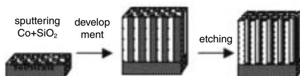
Fig. 1 Metal templating method.
