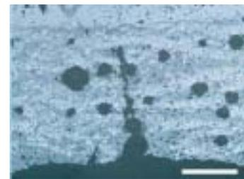
Fig. 4C Small bubbles found in the reaction layer of Zircon. Scale Bar: 1mm
