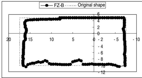
Fig. 3B Measured residual shape of the lower part of L-shaped test piece of FZ-B (mm).
