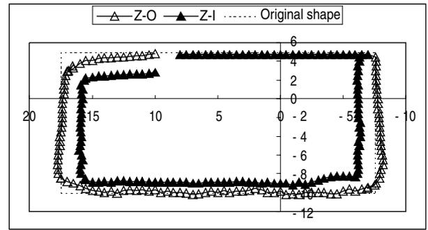
Fig. 4B Measured residual shape of the lower part of L-shaped test piece of Zircon (mm).
