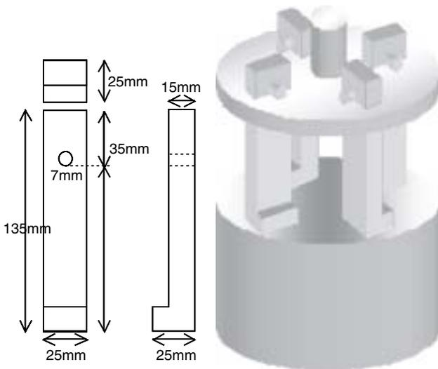
**Fig. 1 L-shaped test piece and the schematic image of the corrosion test.**
