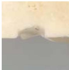
Fig. 3C Upward drilling corrosion formed in WT at the bottom plane of FZ-B.
