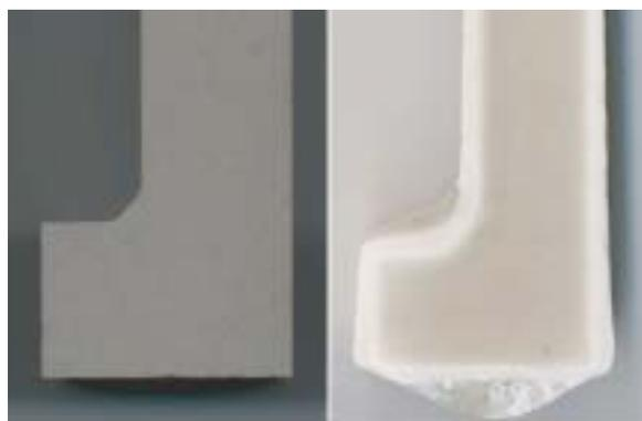
Fig. 4A Cross sections of Zircon before (left) and after (right) the corrosion test.
