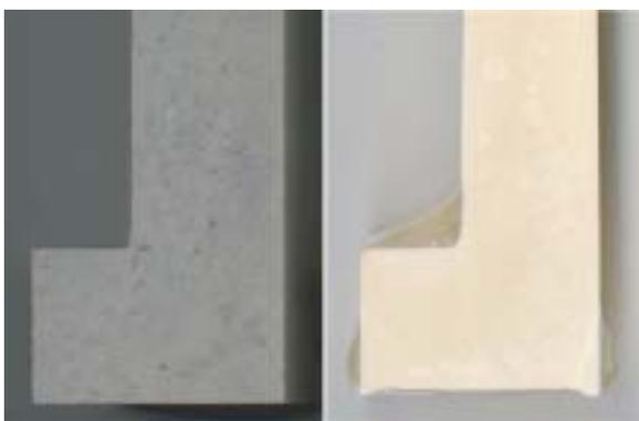
**Fig. 2A Cross sections of FZ-A before (left) and after (right) the corrosion test.**
