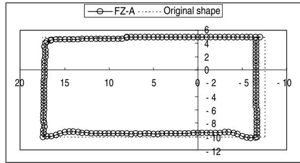
**Fig. 2B Measured residual shape of the lower part of L-shaped test piece of FZ-A (mm).**
