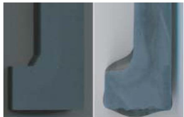
Fig. 5A Cross sections of Tin-oxide before (left) and after (right) the corrosion test.
