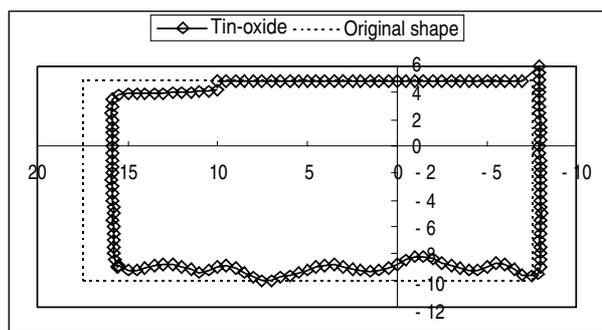
Fig. 5B Measured residual shape of the lower part of L-shaped test piece of Tin-oxide (mm).
