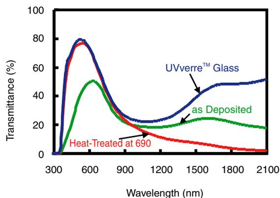
Fig. 2 The transmission spectra of the as-deposited and heat-treated (690 °C) films and a UVverre™ glass substrate. The films were deposited in an Ar gas.
