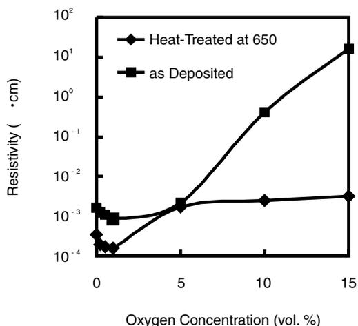
**Fig. 3 The resistivity of ITO films as a function of oxygen concentration in a sputtering gas.**
