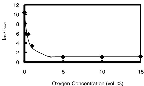
Fig. 8 The ratio of XRD intensities of the (222) plane after to before heat-treatment.
