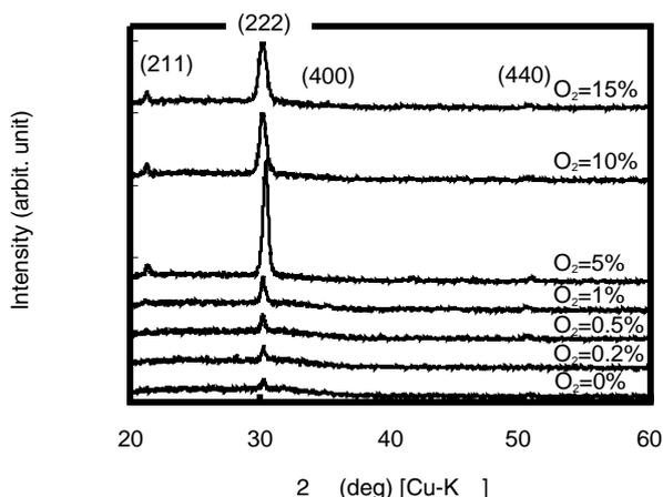
Fig. 6 The XRD patterns of the as-deposited films.
