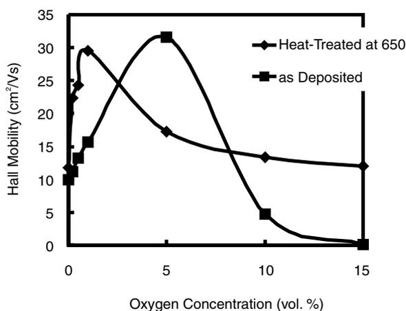
**Fig. 4 The Hall mobility of ITO films as a function of oxygen concentration in a sputtering gas.**
