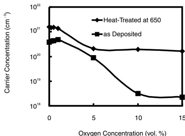
**Fig. 5 The carrier concentration of ITO films as a function of oxygen concentration in a sputtering gas.**
