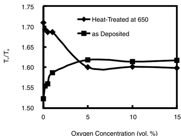
Fig. 1 The  $T_v/T_e$  ratio as a function of oxygen concentration in a sputtering gas.
