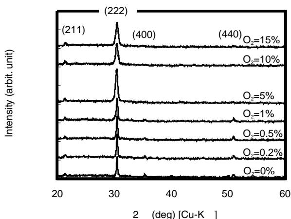
Fig. 7 The XRD patterns of the films heat-treated at 650 °C.
