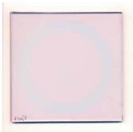
Fig.4 Picture of pink coating glass after Taber-abrasion test.
