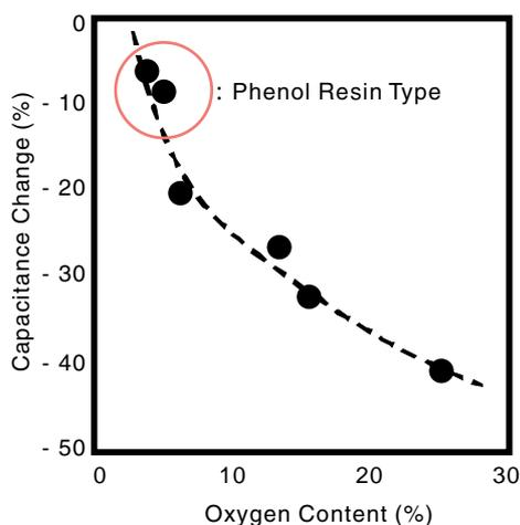
**Fig. 7 Influence of oxygen content of activated carbon used for electrode on capacitance change of capacitor after voltage application of 2.8V at 70 °C for 1000h.**
