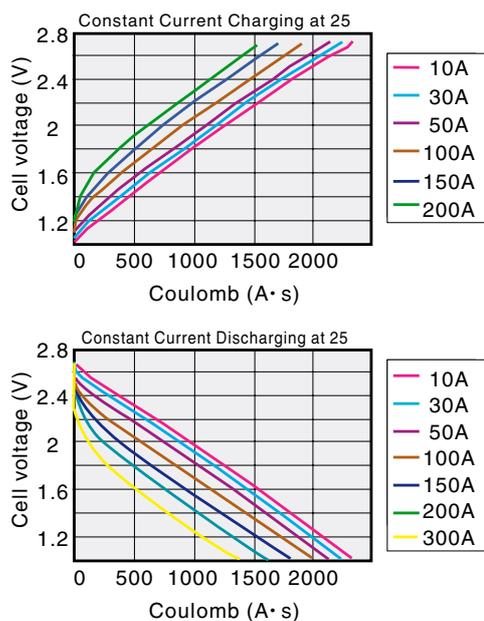
**Fig. 9 Constant current charge-discharge characteristics of DPC14B cell.**
