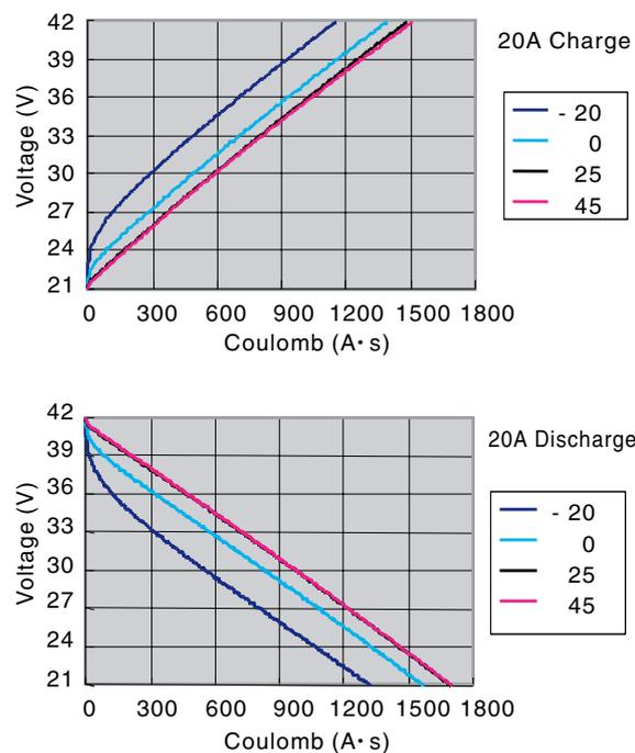
Fig. 14 Temperature dependence on charge-discharge characteristics of ACTC4012-6M3 module.
