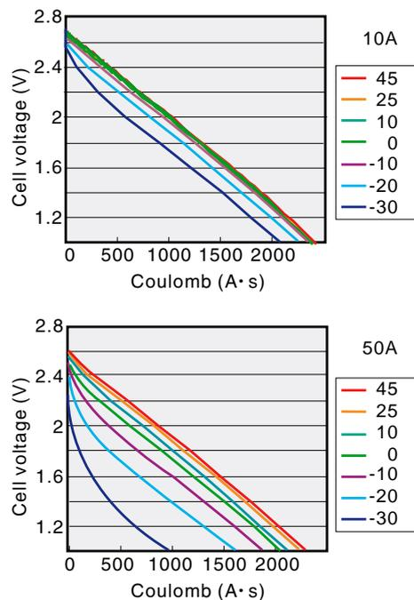
**Fig. 10 Temperature dependence on discharge of DPC14B cell.**
