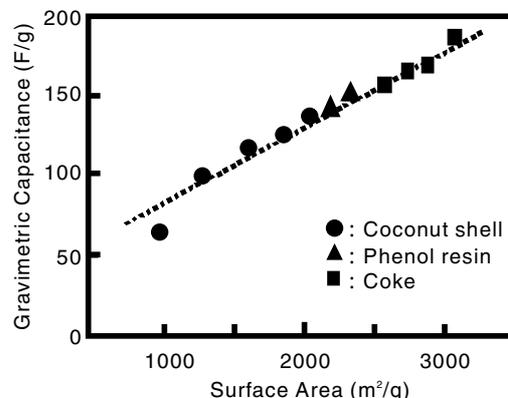
**Fig. 4 Correlation between gravimetric capacitance and surface area of activated carbon.**
