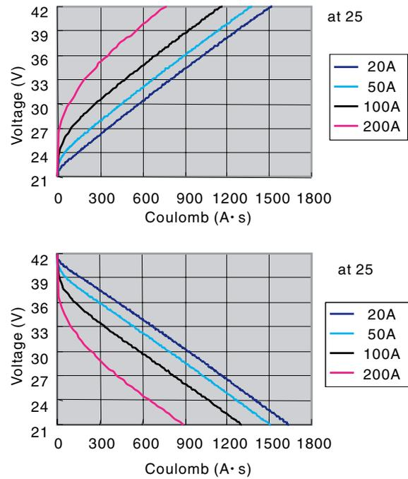
Fig. 13 Constant current charge - discharge characteristics of ACTC4012-6M3 module.
