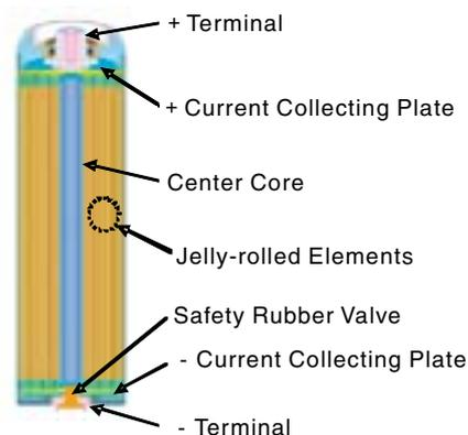
**Fig. 8 New cylindrical cell structure.**
