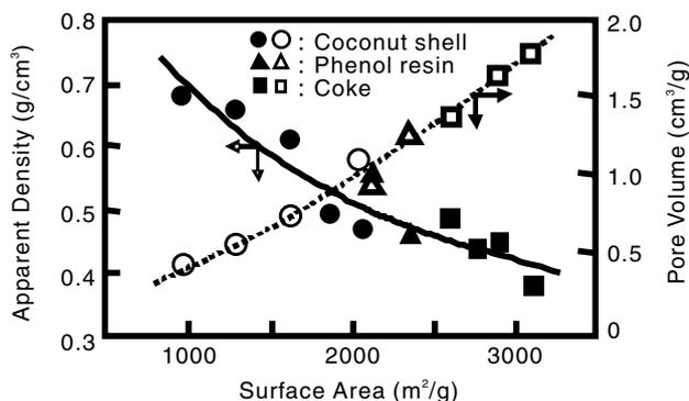
**Fig. 6 Correlation between apparent density of PTFE-bonded activated carbon electrode and surface area of the activated carbon.**
