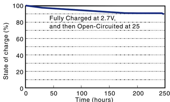
**Fig. 11 Self-discharge performance of DPC14B cell.**
