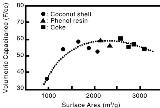
**Fig. 5 Correlation between volumetric capacitance of activated carbon electrode and surface area of the activated carbon.**
