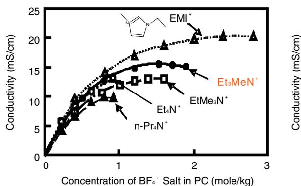
**Fig. 1 Conductivities and solubilities of quaternary ammonium tetrafluoroborate salts in propylene carbonate.**
