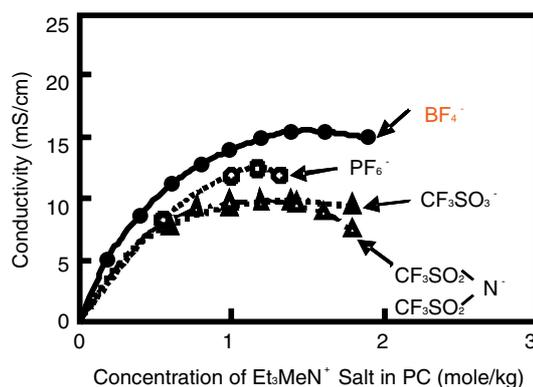
**Fig. 2 Conductivities and solubilities of triethylmethyl ammonium salts in propylene carbonate.**
