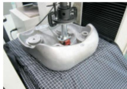
Fig.8 Creep strain examination using hip model.
