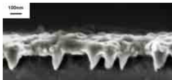
Fig.9 Scanning electron micrographs of Ag thin films on amorphous glass substrates, cross section view after breakage of the sample.
