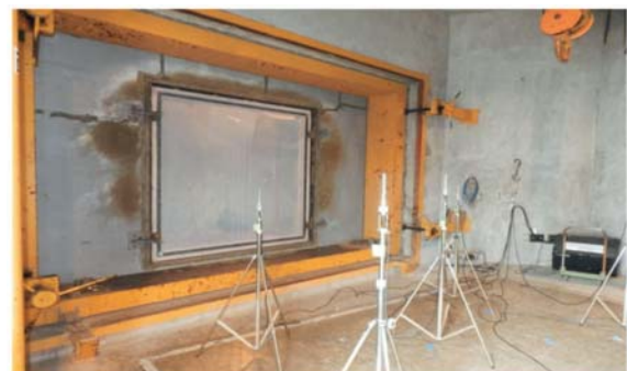
Fig.13 Sound insulation test of the ETFE film
