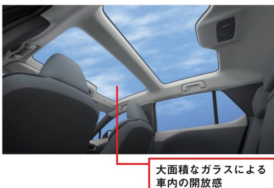
Fig. 1 Panoramic roof glass with Low-E coating of LEXUS RZ<sup>(1)</sup>
