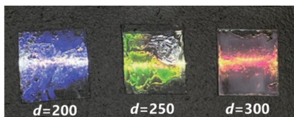
Fig. 3 Appearance of silica-PEG three-dimensional photonic crystal (3DPhC) film with silica diameters d ranging from 200 to 300 nm.
